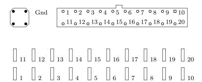
Figure 2: The connector pinout and the geometry of mirror actuators for the 20-ch linear piezoelectric mirror (view from the front side).
