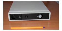
Figure 4: Front and back panels of 20 channel high-voltage amplifier unit.
