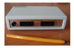
Figure 7: Back panel of the USB control unit with a ground connector.
