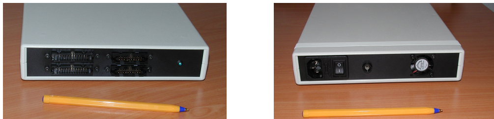
Figure 5: Front and back panels of 40 channel high-voltage amplifier unit.
