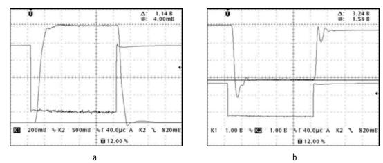
Pumping current pulse (a) and voltage pulse registered in a laser diode bar (b)
