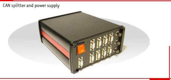
CAN-SPL module provides simultaneous operation of up to 32 PSCM-120 modules while using PTS-U0915 connection cable or 8 modules while using PTS-U0910 cables.
