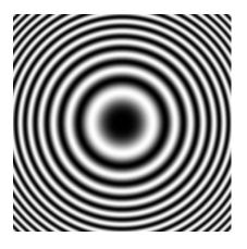
Interference pattern, or Newton's rings, by reflection just above the lens.
